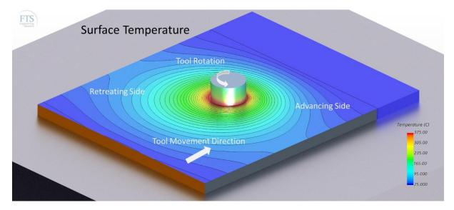
It is important that original joint line is mixed and compressed by the FSW tool during welding, whilst keeping workpiece temperature controlled to avoid the generation of flash at the edge of the workpiece shoulder. Optimised welding procedures can be developed by welding trials, but there are significant advantages associated with the use of an accurate computer model to develop robust welding procedures.
