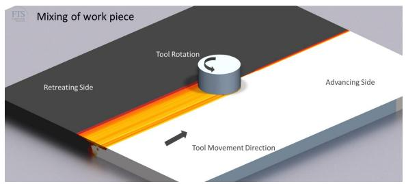
A computer model of FSW can be used to make sensitivity studies of tool shapes before welding trials and to investigate the effect of variations in workpiece properties that may not be possible in a small welding trial. The methods developed by Oxcam Engineering Arc can be used in a straightforward manner to reduce the costs associated with the implementation of FSW within the requirements of new industrial applications.
